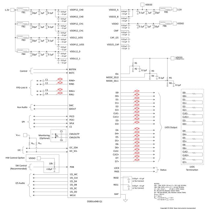
Figure 8-2. Typical Connection Diagram (STP)
