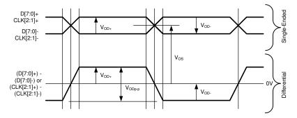
Figure 6-9. FPD-Link Single-Ended and Differential Waveforms
