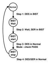
Figure 7-13. BIST Mode Flow Diagram
