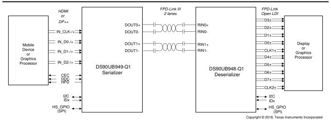
Figure 8-3. Typical Display System Diagram
