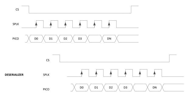
Figure 7-2. Forward Channel SPI Write
