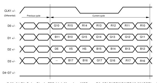
Figure 7-20. 24-Bit Color Single FPD-Link Mapping: MSBs on D3, "OLDI/SPWG/VESA" (MAPSEL = H)
