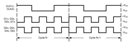
Figure 6-1. Checkerboard Data Pattern
