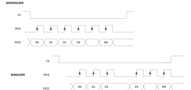
Figure 7-4. Reverse Channel SPI Write
