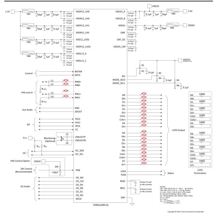
Figure 8-1. Typical Connection Diagram (Coax)
