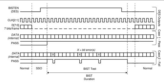
Figure 7-14. BIST Waveforms
