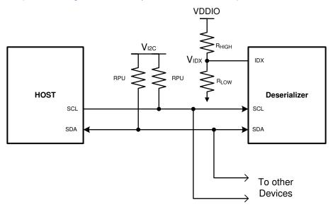
Figure 7-28. Serial Control Bus Connection
