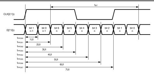
Figure 6-10. FPD-Link Transmitter Pulse Positions
