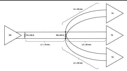
Figure 7-12. FPD-Link Fan-Out Electrical Requirements
