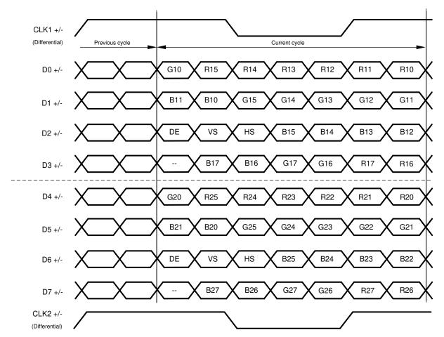
Figure 7-18. 24-Bit Color Dual FPD-Link Mapping: MSBs on D3/D7,"OLDI/SPWG/VESA" (MAPSEL = H)
