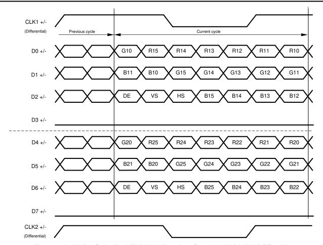
Figure 7-23. 18-Bit Color Dual FPD-Link Mapping, Standard 18 Bit (MAPSEL = L)
