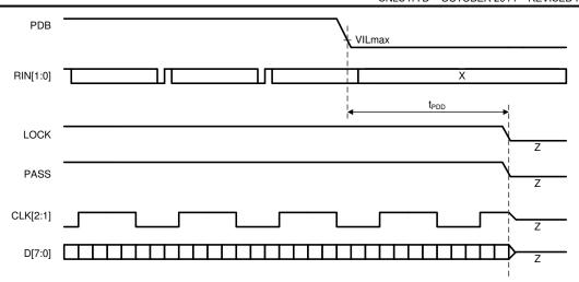
Figure 6-5. FPD-Link and LVCMOS Power Down Delay
