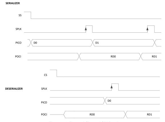
Figure 7-3. Forward Channel SPI Read
