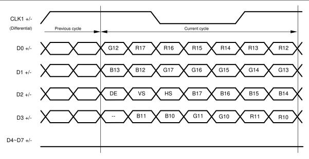
Figure 7-21. 24-Bit Color Single FPD-Link Mapping: LSBs on D3, "JEIDA" (MAPSEL = L)
