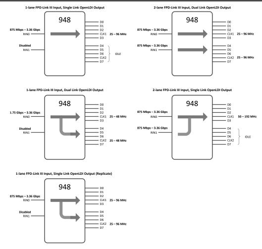
Figure 7-15. Data-Path Configurations
