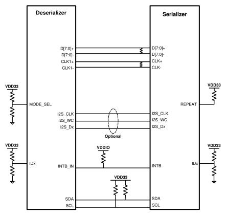
Figure 7-11. Repeater Connection Diagram
