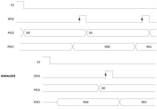
Figure 7-5. Reverse Channel SPI Read
