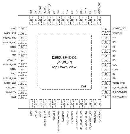
Figure 5-1. NKD Package 64-Pin WQFN Top View
